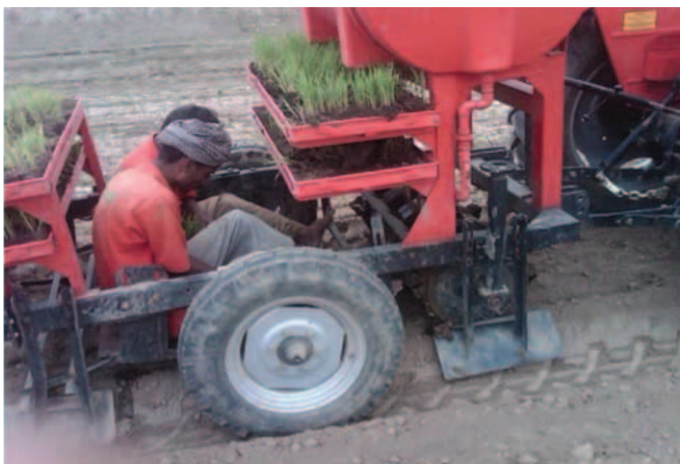
Figure 45: Machine carrying laborers who drop 10-day-old seedlings into holes punched by the machine as it moves along the beds.
